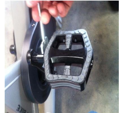
Tightening the Pedals Tool: 15mm Open Ended Wrench
