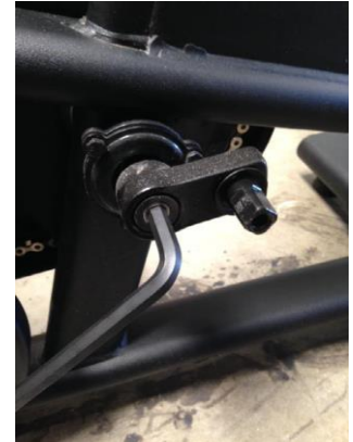
Bell Crank Fixing Bolts Tool: 8mm Hex Wrench
