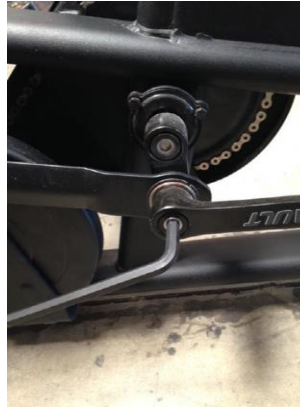
Crank Fixing Bolts Tool: 8mm Hex Wrench
