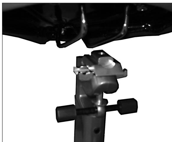
Loosen the seatholder locking screw and turn the upper locking lever so that it is aligned with the equipment. Place the seat into position on the grooves of the lower locking lever. Turn the upper locking lever towards the top of the seat rails and lock the seat by tightening the locking screw.
