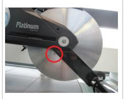
fit the sensor bracket to the chain cover in a possition where the magnet passes for speed pickup. put the sensor in the holder.
