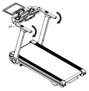
Connect the power cable (C15) and insert the safety key (C13).
