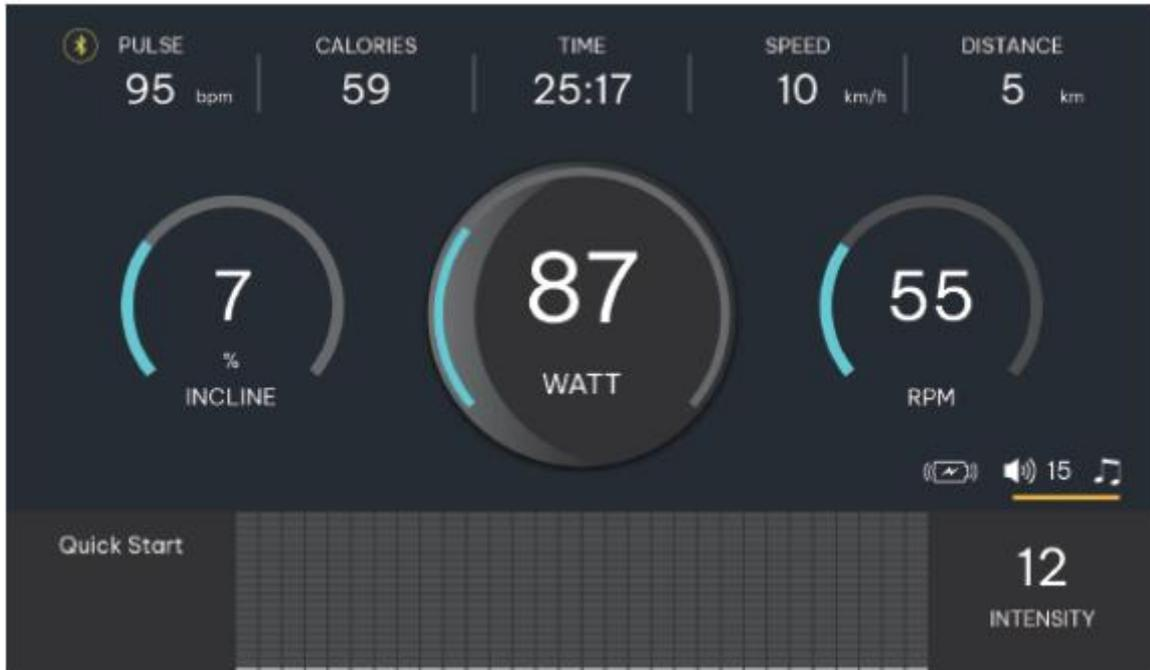
**PULSE:** If you wear the chest belt or hold the pulse sensors on the handles, the pulse rate will be displayed
