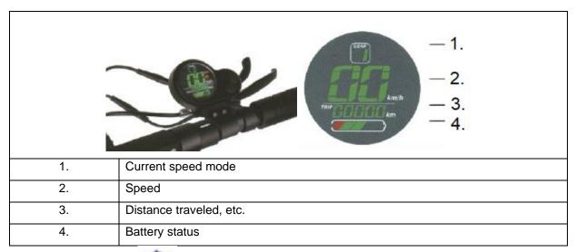
Hold the power button for 3 seconds to turn on. The LCD display enters standby mode.
