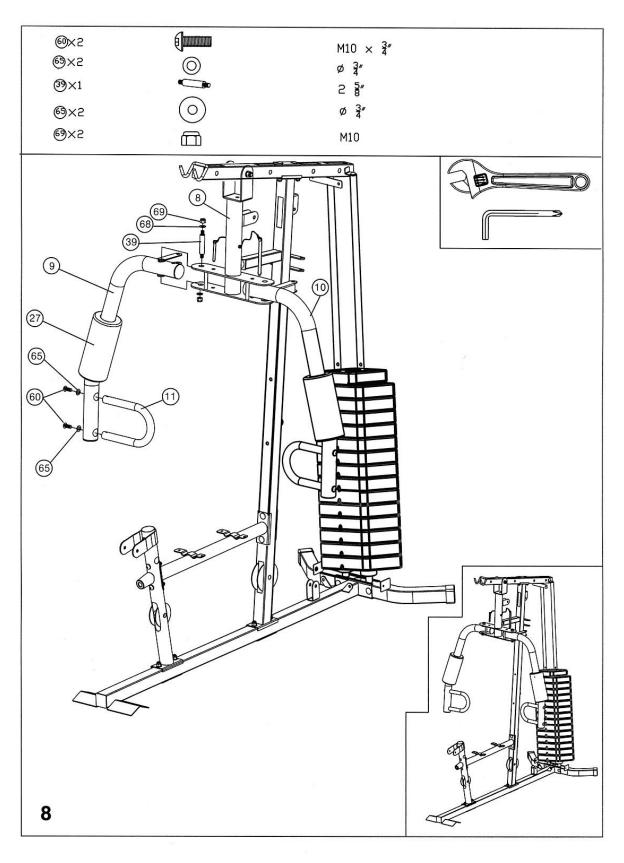
Attach the right (9) and left (10) butterfly arms to the butterfly base (8) using the 2x axles (39), 4x washers (68) and 4x nuts (69). Slide the foam rollers (27) and then the handles (11) onto the arms (9) and (10) using 4x washers (65) and 4x bolts (60).
