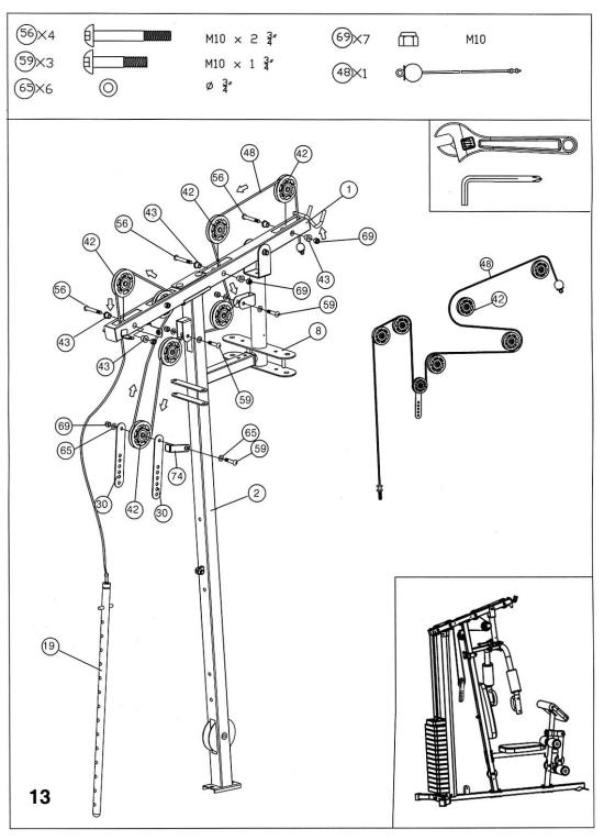
Pass the cable (48) and attach the threaded end to the weight selection rod (19). Attach 4x pulleys (42) to the top frame (1) with 4x bolts (56), 8x bearings (43), and 4x nuts (69).
