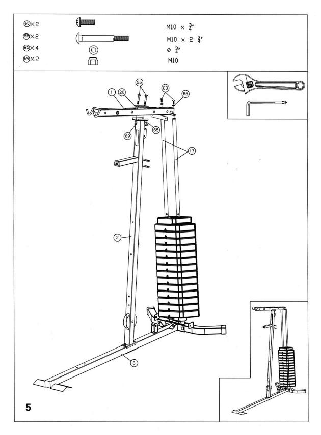
Attach the top frame (1) to the vertical frame (2) using 2x washers (65), 2x nuts (69), bracket (20) and 2x bolts (55). Attach the top frame (1) to the guide bars (17) with 2x bolts (60) and 2x washers (65).
