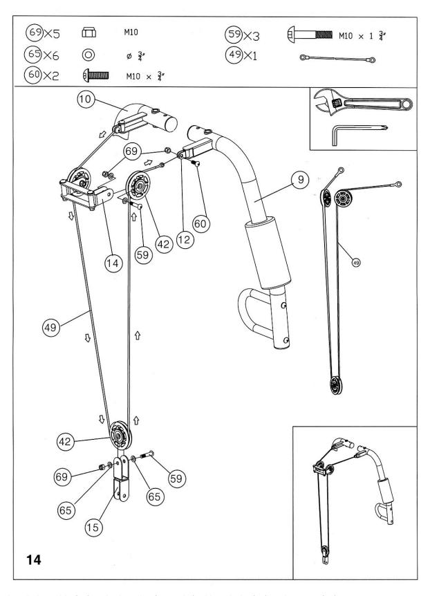
Attach the cable (49) to the handles (10 and 9) with 2x bolts (60) and 2x nuts (69). Attach 2x pulleys to the pulley holder (14) with 2x bolts, 4x washers (65) and 2x nuts (69).
