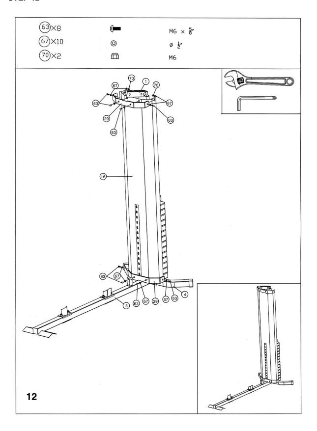
On the top, attach the cover (16) to the upper frame (1) using the cover bracket (29), 4x bolts (63), 6x washers (67) and 2x nuts (70).
