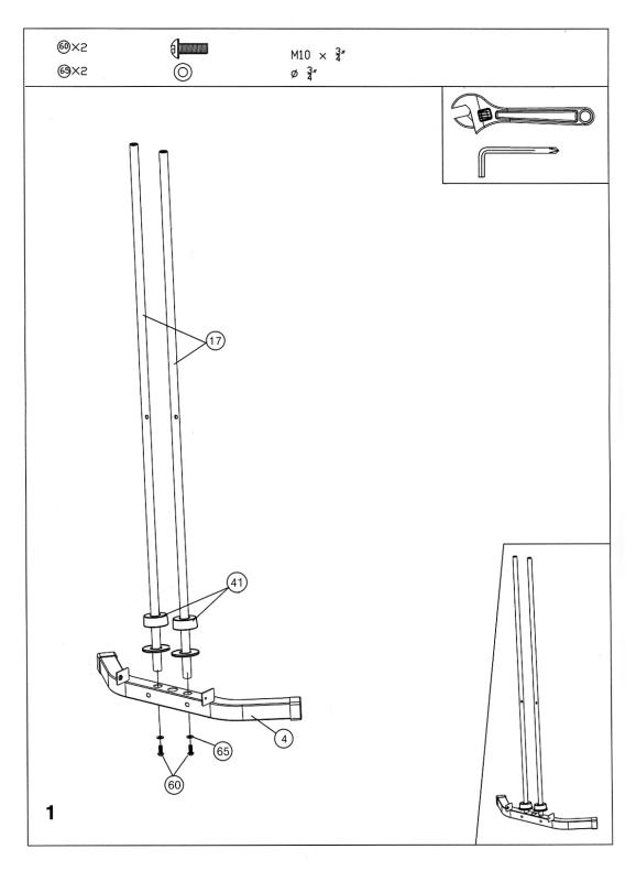
Attach the guide rods (17) to the rear stabilizer (4) with 2x bolts (60) and 2x washers (65). Slide the rubber washers (41) onto the rods.
