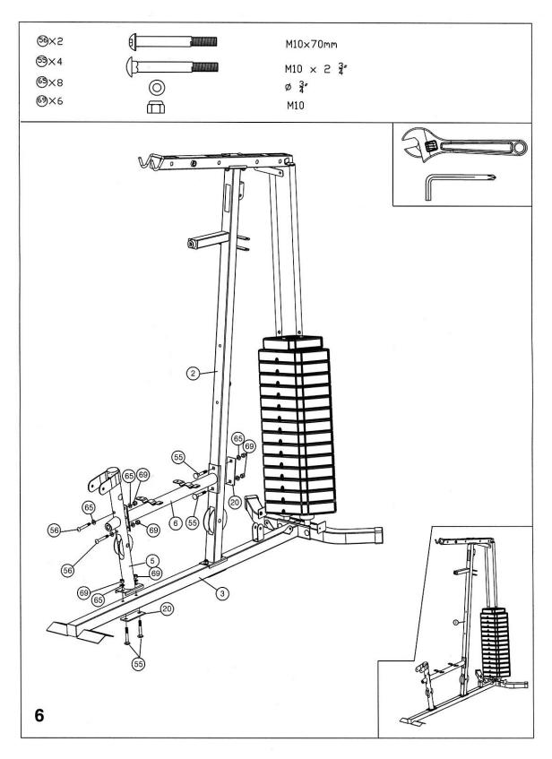
Attach the saddle frame (6) to the vertical frame (2) using the plate (20), 2x washers (65), 2x nuts (69) and 2x bolts (55). Attach the leg press holder (5) to the base (3) using the plate (20), 2x bolts (55), 2x washers (65) and 2x nuts (69). Attach leg press holder (5) to the saddle frame (6) using 2x nuts (69), 4x washers (65) and 2x bolts (56).
