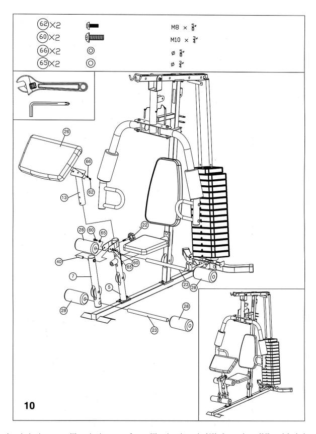
Attach the leg press (7) to the leg press frame (5) using the axle (40), 2x washers (65) and 2x bolts (60). Attach the arm curl stand (13) to the leg press holder (5) and secure with the knob (22). Attach
