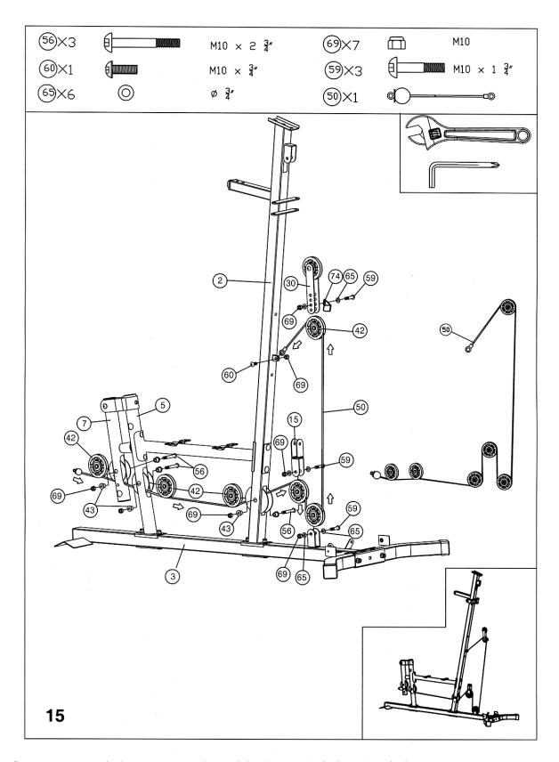
Secure the cable (50) to the vertical frame (2) with the bolt (60) and nut (69).
