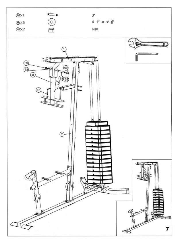
Attach the butterfly base (8) to the top frame (1) using the axle (38), 2x washers (68) and 2x nuts (69). Secure the frame (8) with the pin (46) when not in use.
