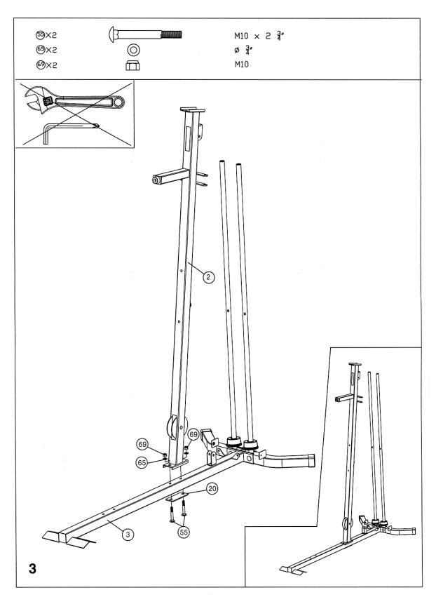
Attach the vertical frame (2) to the base (3) using the plate (20), 2x bolts (55), 2x washers (65) and 2x nuts (69).
