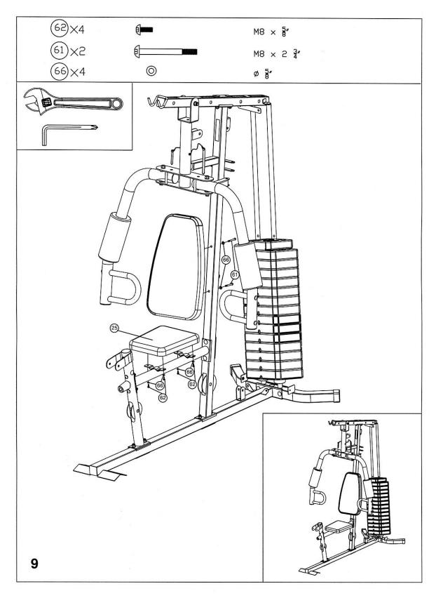
Attach the backrest (24) with 2x bolts (61) and 2x washers (66). Attach the seat (25) with 4x washers (66) and 4x bolts (62).
