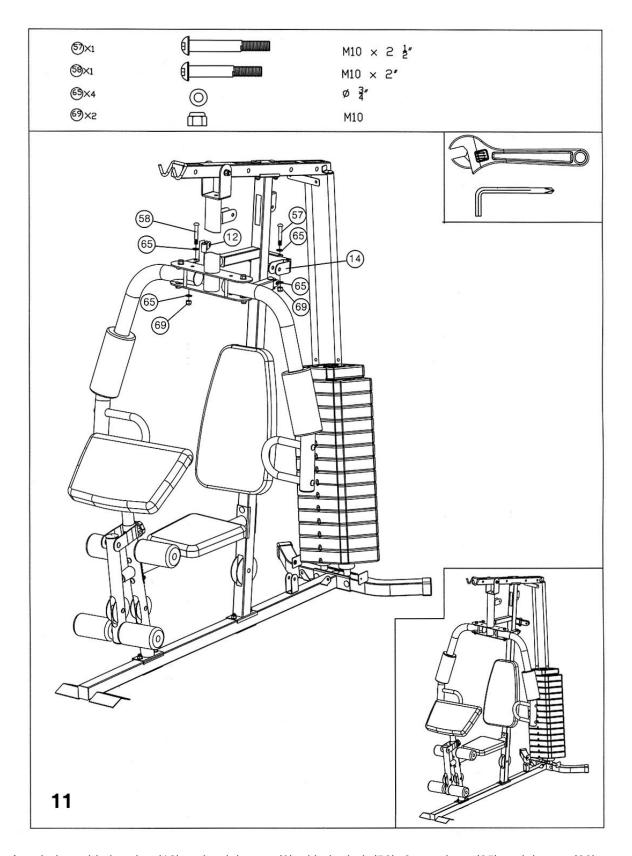
Attach the cable bracket (12) to the right arm (9) with the bolt (58), 2x washers (65) and the nut (69).
