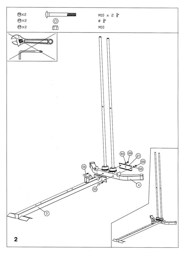
Attach the rear stabilizer (4) to the base (3) using the plate (21), 2x bolts (55), 2x washers (65) and 2x nuts (69).
