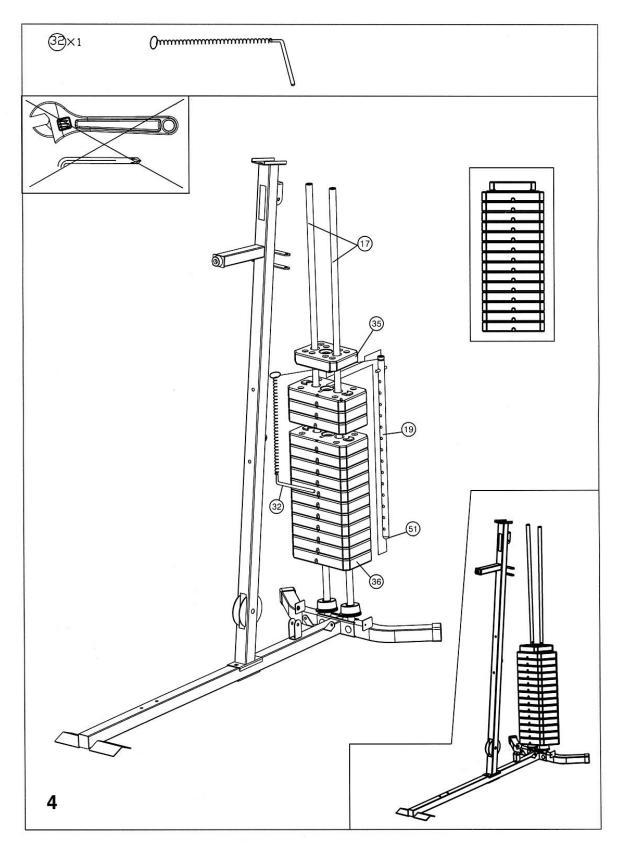
Slide the weights (36) onto the guide rods (17), slide the end cap (51) and then slide the weight selection rod (19). Attach the weight selection pin (32) to the guide bar and then to the weight. Slide the upper top weight (35).
