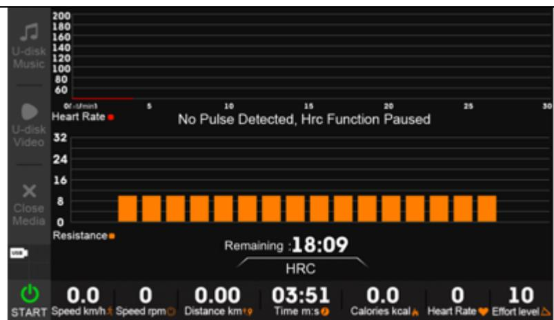
If no pulse is detected, the following screen is displayed.
