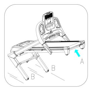
Before attempting to move the treadmill, please make sure the treadmill has been properly folded and the power cord has been removed from the outlet.
