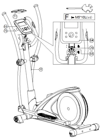
Connect the computer cable (29) and cable of hand pulse cable (65) with the computer (64), then fix the computer (64) on the handlebar post (10) by using the screws (76).
