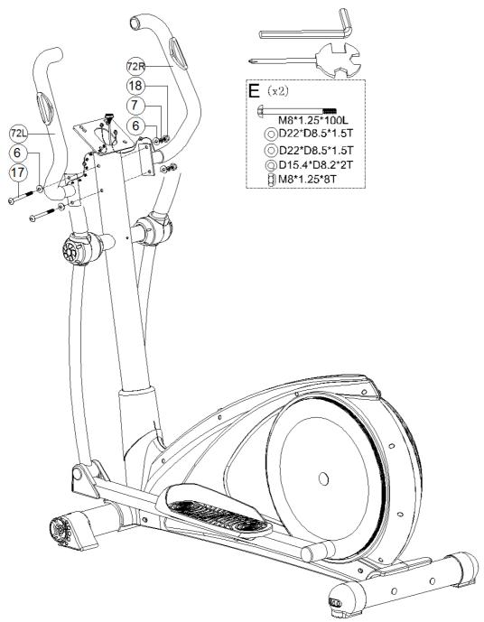
Assemble the left and right fixed handlebar (72L &72R) on the handlebar post (10) by using the Allen bolt (17), the curved washer (6), the spring washer (7) and the domed nut (18).
