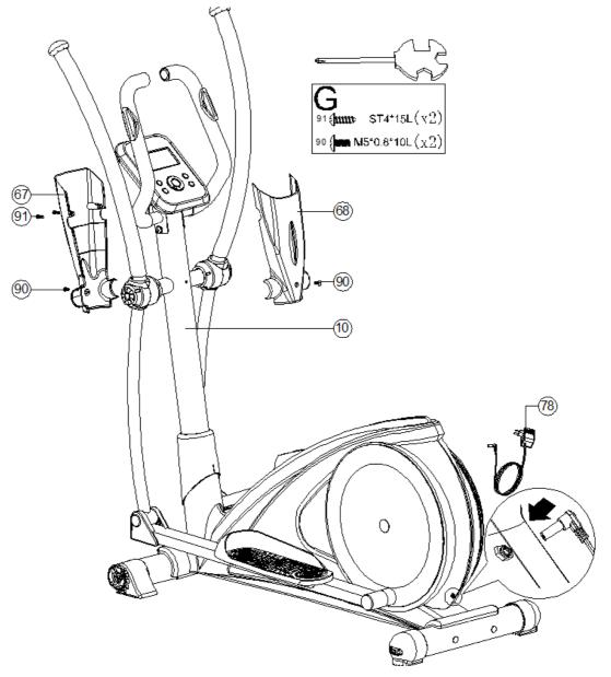
Fix the front computer cage (68) & rear computer cage (67) on the front post (10) using screws (90&91). Insert the adaptor into the electric socket when exercise.
