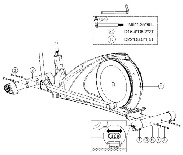
Assemble the front stabilizer (2) and rear stabilizer (19) onto the main frame (1) by using the inner Allen bolt (3), the curved washer (6) and the spring washer (7).
