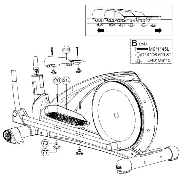
Assemble the left and right pedal (21L&21R) on the pedal supporting tube (11) by using the square neck bolt (20), flat washer (73) and knob (77).
